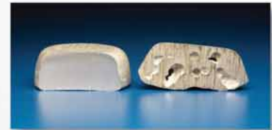
Degassing virtually eliminates porosity in the casting.
