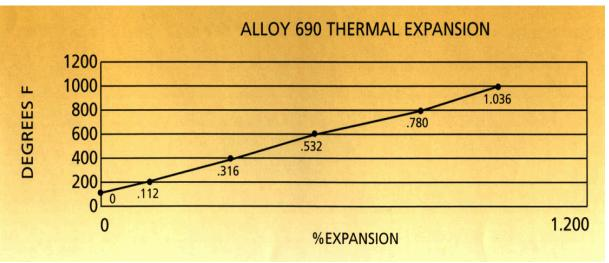
Test conducted in accordance with test Specification ASTM E-228. Sample size of 0.25 inches in diameter by 2.00 inches long.
